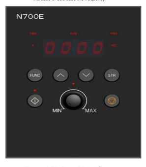
Fig.4-1 LED Type Digital Operator
